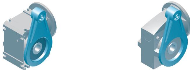
The torque arm is a compact and simple method for absorbing reaction torques with shaft-mounted gear units. The torque arm is mounted on the B14 threaded holes of the NORD UNIVERSAL worm gear unit and can be installed with rotation steps of 45°.
