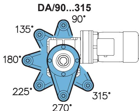
The torque support can be mounted in 45° steps to the angles 90 - 315 both on output side A and output side B.
