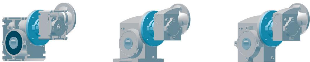
The double worm gear adapter enables the connection of two NORD UNIVERSAL worm gear units to form a double worm gear unit. The double worm gear units can be installed as both angular gear units or as parallel axis units.
