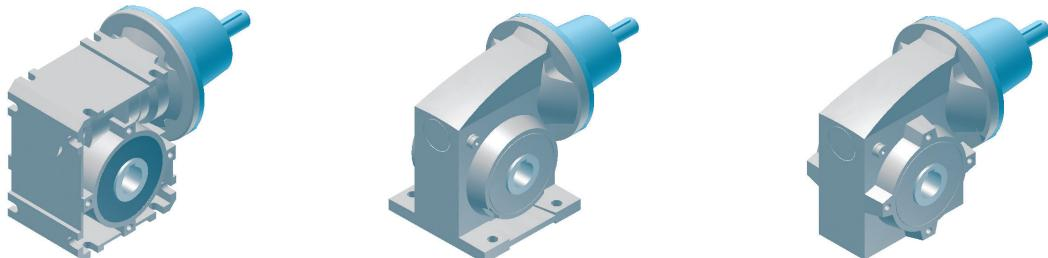
The Type W free input shaft was developed to attach couplings, belt pulleys or chain wheels to the input of NORD UNIVERSAL worm gear units. The Type W free drive shaft is available for sizes 40, 50, 63 and 75. The components includes the pre-assembled, lubricated-for-life unit, the coupling sleeve and all the necessary fastening elements.
