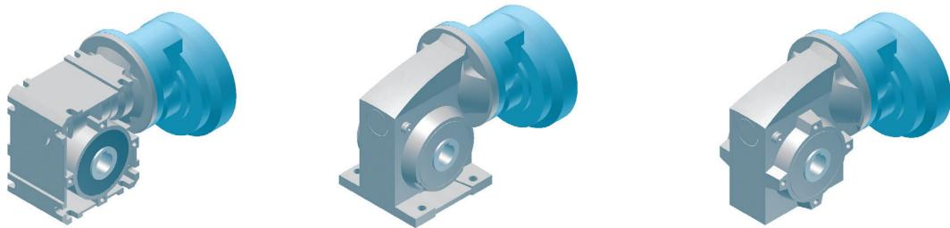
With the H10 helical gear input, the NORD UNIVERSAL worm gear unit is converted into a 2-stage helical worm gear unit. The speed ratio of the H10 helical gear is the same for all sizes, namely  $i_{vor} = 10$ .
