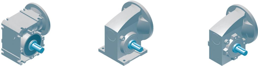
The plug-in shaft V (single side plug-in shaft) are plugged in to the standard hollow shaft of the NORD UNIVERSAL worm gear unit and axially secured. The standard journal dimensions for the individual sizes are shown in the following table. The tolerance of the free shaft journal is h6 for all units.
