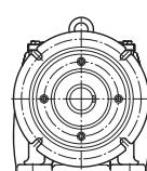
Housing in foot mounted design with Flange B5
