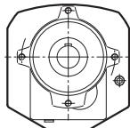
Housing in flange mounted design with Flange B14
