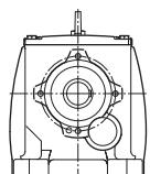
Housing in foot mounted design with Flange B14
