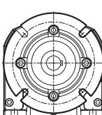
Housing in foot mounted design with Flange B5
