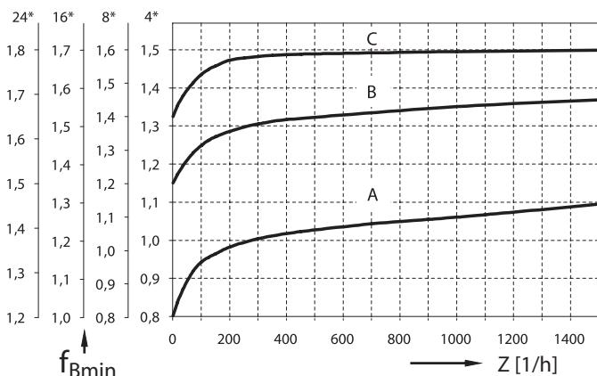
Diagram 1: Minimum service factor  $f_{B\min}$
