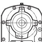
Housing in foot mounted design with Flange B14
