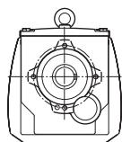
Housing in flange mounted design with Flange B14
